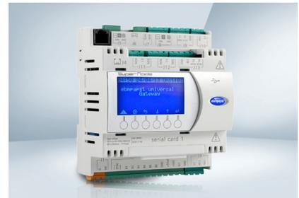
The ebm-papst Universal Gateway enables communication between MODBUS fans and other protocols used in a building management system, e.g. BACnet. One of its distinct advantages is its high level interface access to all AHU fans, meaning that every fan can be monitored and controlled independently. This also enables closed-loop pressure control and monitoring of all fans in real time.
